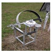
Recent data streams from Macquarie University (MQ) have indicated consistent close matching of Diffuse and Global irradiation measurements suggesting a continuously overcast but luminous sky or, more likely, that the shadow band on the Diffuse Radiometer (pictured) is out of adjustment. Accordingly, we are using
